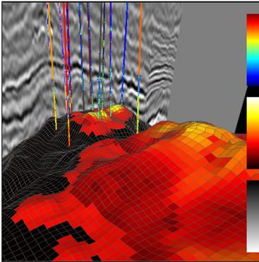
3D view of oil saturation simulation and 3D seismic data for reservoir monitoring
