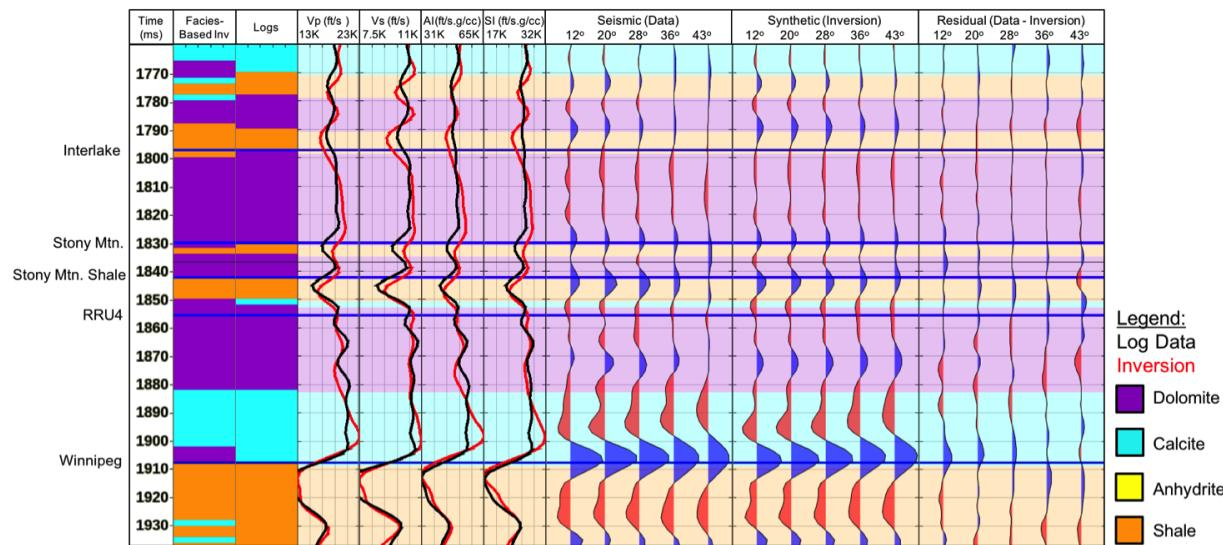
Figure 3: Well A facies-based inversion elastic properties results. Log data in black, and inversion results in red. Track 1 displays output facies results from inversion while track 2 shows well log facies (data). Refer to Figure 1 for well location.
