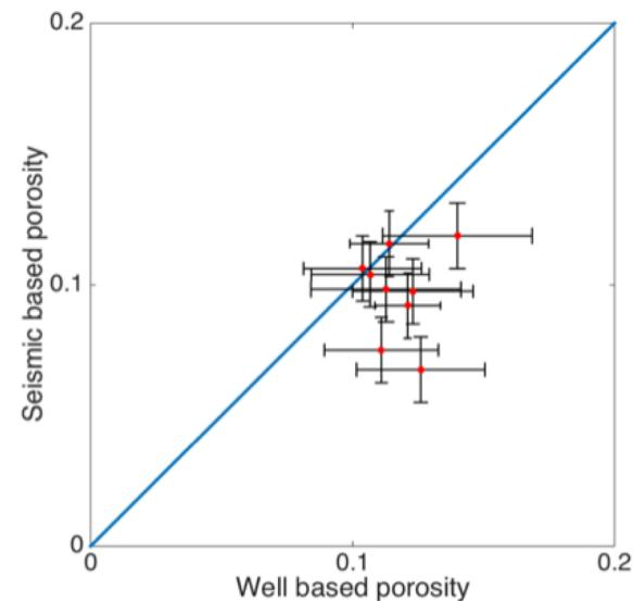
Figure 7: RRU4 seismic derived porosity versus porosity from well data. Red dots represent 9 wells within field unit. Porosity value at each well correspond to the mean log value (red dot) for RRU4 interval and uncertainty bar (horizontal) is the standard deviation. Seismic derived porosity is extracted at corresponding well location with 2.5 p.u. uncertainty bar width (vertical). Blue line represents the 1:1 line.
