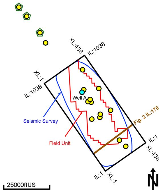
Figure 1: Available dataset include 44 mi<sup>2</sup> seismic dataset (blue polygon) and 17 wells (dots). Green pentagon corresponds to wells with dipole sonic. The field unit outline (red) defines all subsequent seismic extractions and well extraction in Figure 3 is from well A in cyan color.
