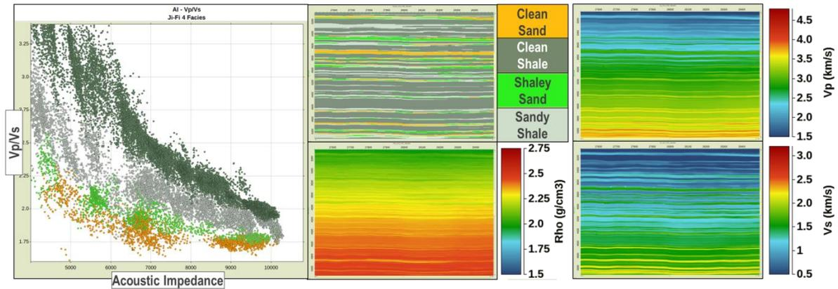
Figure 3: Comparison of reference (top) and inversion result (bottom): AI-Vp/Vs crossplot and section views of Facies, Vp, Vs, Density. Intercept and gradient equivalent seismic properties (AI-Vp/Vs) are distributed correctly in the inversion results without the classic averaging artifacts seen in facies unaware inversions. Facies, Vp, Vs, and Rho values are sensible.
