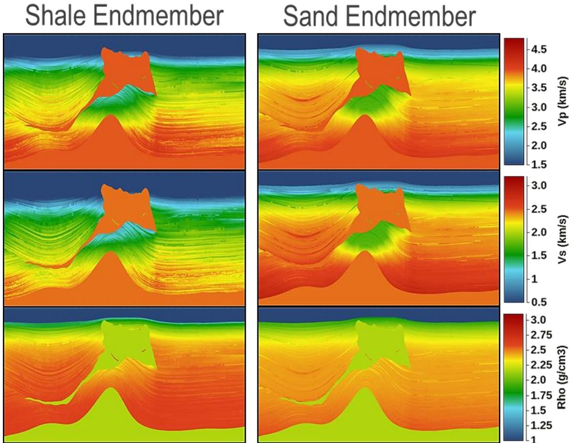
Figure 1: Endmember shale (right) and sand (left) Vp-Vs-Rho values. The two models consider pressure, porosity, temperature, and mineralogy. The area under the salt intrusion tends to have higher porosity and increased pore pressure. To the right of the salt intrusion, the model contains areas of over- and under-pressure.
