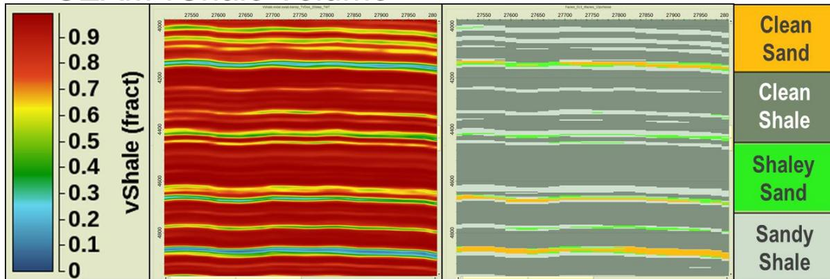
Figure 4: Detailed image of vShale volume (left) and inversion results (right). Thin, sandy shale beds have been identified and subtle sand-shale variations are nicely captured in the joint facies inversion.
