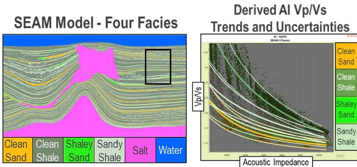
Figure 2: Facies and inversion window (left) and AI- $V_p/V_s$  crossplot of properties modeled over the inversion window. Lines indicate the mean trend and uncertainties for each facies. Uncertainties for each facies were determined using a pseudo-well passing through the center of the inversion window.
