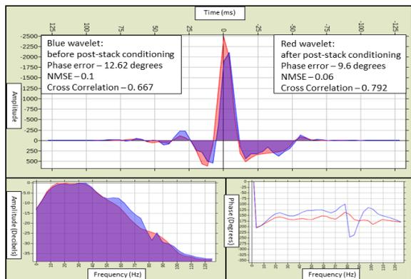
Figure 3b: Wavelet comparison using the 'Roy White method' before and after post-stack SDC where the wavelet has smaller side lobes, reduced phase error, decreased NMSE (Normalised Mean Square Error) and a higher cross-correlation coefficient when compared to well synthetics and seismic data.
