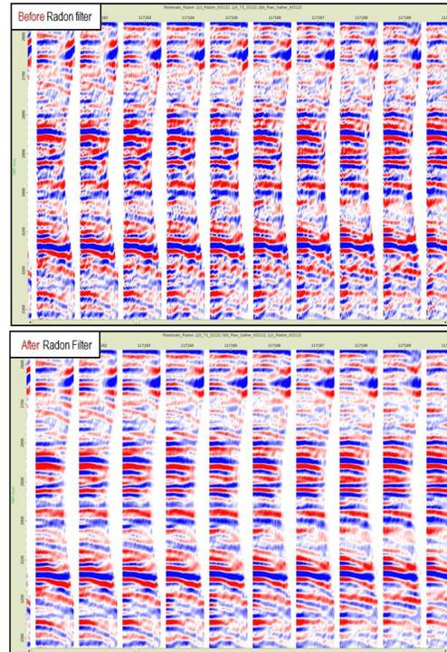
Figure 1: High resolution Radon demultiple applied to a North Sea seismic dataset.
