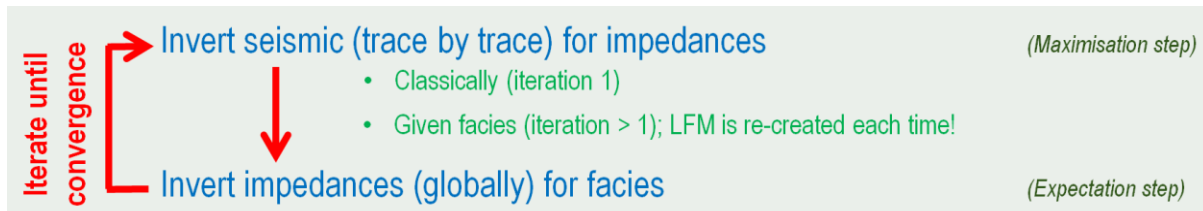
Figure 1 The Expectation-Maximisation method. In iteration 1 of the Maximization step, the LFM is the membership weighted average of the input LFM's. The misfit between synthetic and seismic is determined as part of the Maximisation step. In the Expectation step, a 3D discrete Markov random Field is used, in which spatial information is embedded; this makes the approach a geostatistical inversion system (as well as a Bayesian one). Note though that variography is not used (not recommended for discrete quantities).
