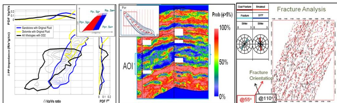
Figure 4. Examples of unconventional reservoir saturation, porosity, and fracture predictions (Malaver et al, 2004; Hardy, 2013; Emsley et al, 2012; Mildren et al, 2013)
