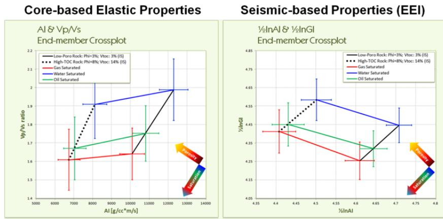
Figure 2. Example of core and seismic end-members as reservoir quality indicators in a tight gas shale play (Malaver, 2013)
