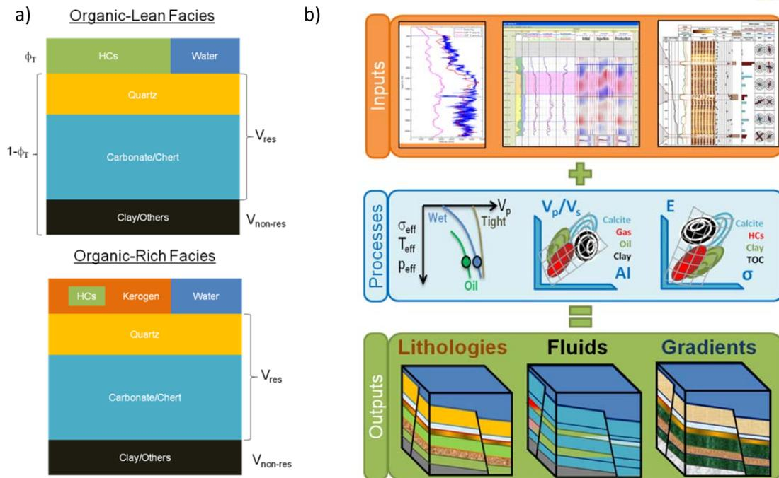
Figure 1. Unconventional reservoir models (a) and a typical Integrated Geoprediction workflow (b)
