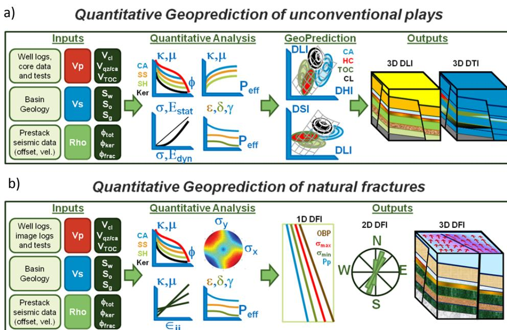
Figure 3. Quantitative Geoprediction workflows for (a) unconventional plays and (b) natural fractures
