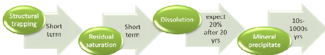
Figure 1: Both the proportion of CO 2 & the security of that stored volume increases with time (left to right) from an injected fluid to a mineral precipitate
